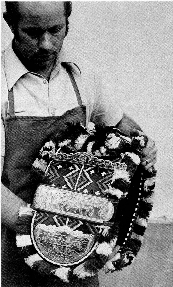
It takes some 25 hours of meticulous work to finish one of the bell straps with leather laces, woollen frills and brass engravings.
