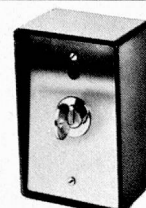
KS531. 3-pole 4 way 5 amps at 300 VAC/DC.
