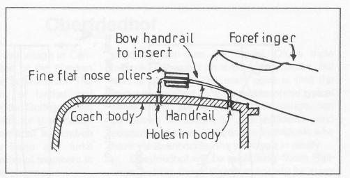
a safe but readily accessible place on the bench. You then place the coach on the bench with one side uppermost, with one door dead in front of you, the coach lying parallel to the edge of your working area. Take the pliers and grip the first handrail at the extreme far end. Now put the other leg into the hole nearest yourself. Place your spare forefinger over the leg you have just inserted and gently bow the handrail so that the other leg goes in. Repeat for the second handrail.
