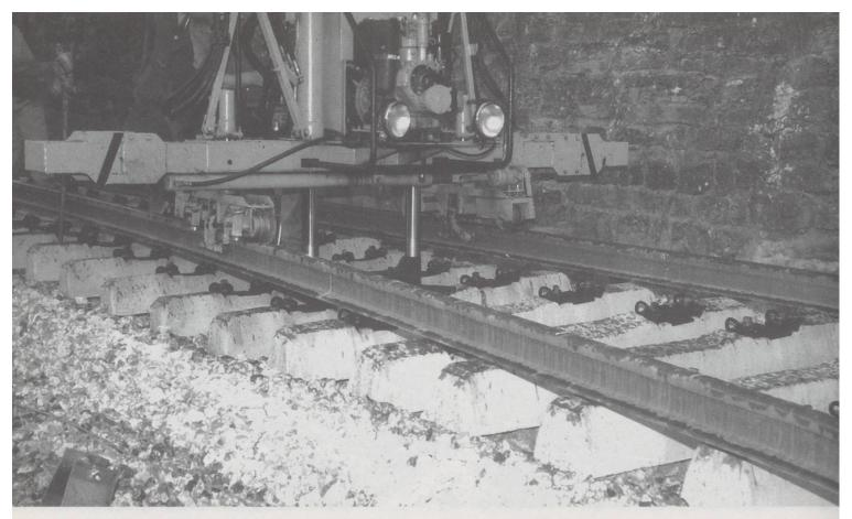
Above: The small machine uses hydraulics to lift the rails onto the metal chairs.
