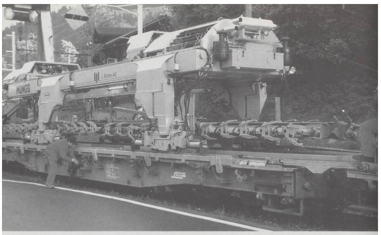
Above: The crane with the lifting spar the fork arms swivel down to pick up the new sleepers.
