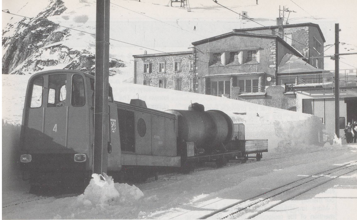
Above: The ex Brienz Rothorn diesel seen here at the summit of Rochers de Naye with a service train taking water to the restaurant, now Hm2/2 4 of the Montreux-Territet-Glion-Rochers de Naye (MTGN) 6th December 1996.
