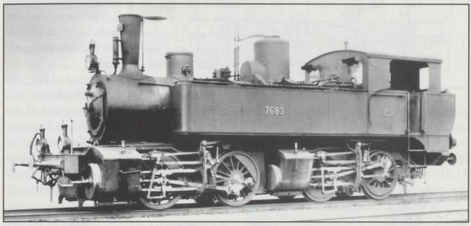
The SCB had need of a locomotive to act as a pilot on passenger trains and to operate freight services from Sissach to Olten over the Hauenstein line with its ruling gradient of 27 per mille. The locomotives under consideration were the 87 tonne D6 2 x 3/3 as built for the Gotthardbahn at a cost of SFr 90 000 or the newly designed C4 2 x 2/2 at a cost of just over SFr 73 000. The SCB chose the latter design and placed an order with Maffei of München for 6 locomotives.
