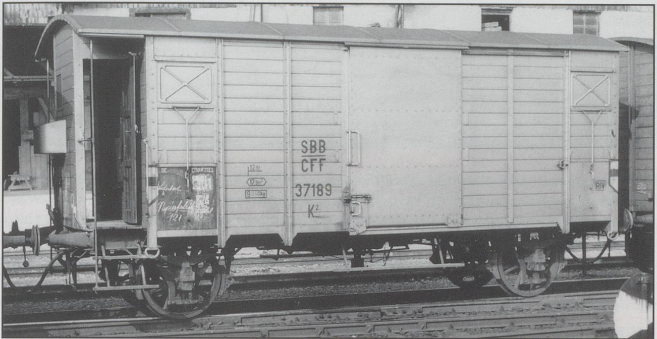
More K 2 vans were built than any other type of goods vehicle in Switzerland. This example, 37189, was photographed at Zürich in 1955. Instead of the usual grey livery, this vehicle had been painted white. Photograph courtesy Eisenbahn Amateur .
