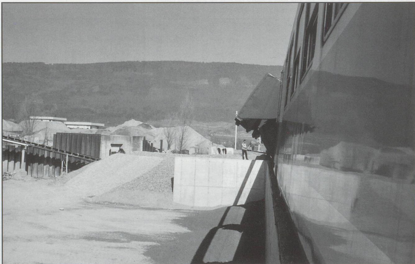
PHOTO 7: The end of the line: the hoppers are unloaded at the works at Sutz. The driver of the train can be seen operating the hoppers by handheld controller. He gets instructions on the radio from the works supervisor about exactly where to unload. No extra staff are needed. After the unloading process is completed, he informs the supervisor by radio, walks to the railcar on the other end and informs the rail dispatcher he is leaving the site. When the train gets back to the main line, access is again controlled in the normal way by a signal.
