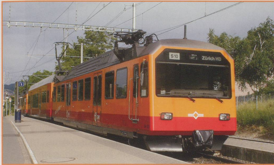
Zürich service at Triemli. Note the offset pantograph
