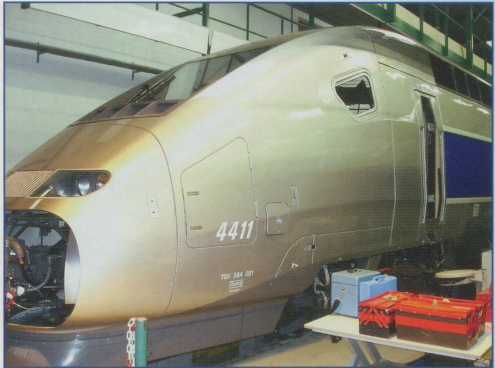
The new 325 kph (= 200 mph) stock, standing in the final testing hall, just before running trials. To cope with this speed, the nose has to be longer and smoother than the previous models.
