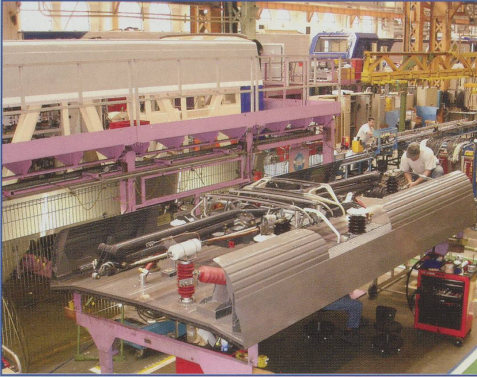
In one of the large halls, different body parts are resting on assembly jigs. The jigs are painted violet, so nobody inadvertently installs anything onto it by mistake! One of the trolleys for the parts can be seen on the right. The jigs are just so high that installation can be done as comfortably as possible - in this case sitting down.
