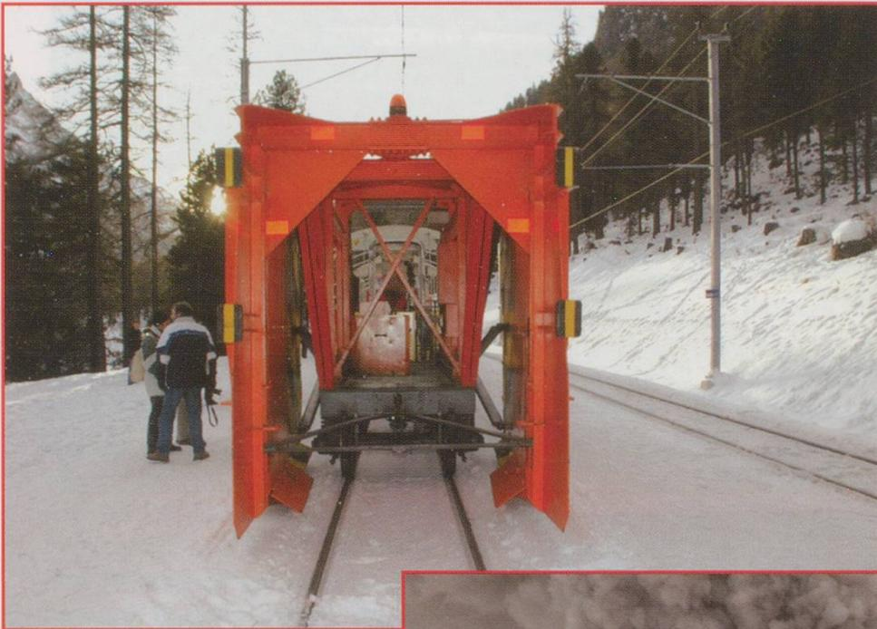
This snow spreader is used on the RhB to assist in winter clearance work after a heavy snow fall. The vehicle has movable wings and is used to set the width of the path through the snow. It is pulled at the end of a works train to cut and funnel the snow to an area where it can be blown with the snow blower.
