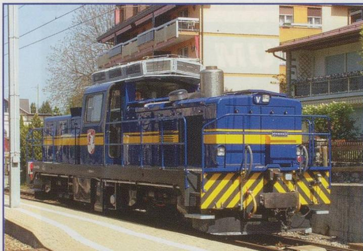
Monday 5th May saw the roll-out of MOB diesel-electric locomotive Gm4/4 No.2004 *Albeuve* after a major overhaul. Built in France by Gaston Moyse of La Corneuve, this loco entered service in 1982, six years after its sister No. 2003 *Montbovon*. These powerful diesels are used for works trains and can also haul passenger stock if there is a problem with the catenary.
