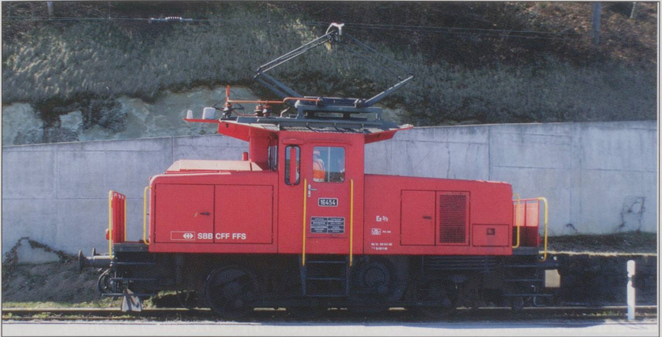
The works still justify a full-time Ee3/3 shunter seen here on the highway crossing outside the works...
