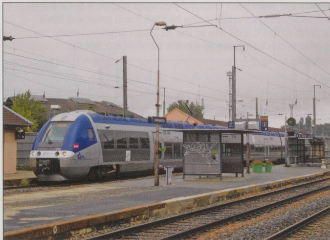
SNCF TER unit at Annemasse Station. This will be much busier once the line is opened in 2019. A new island platform will be built to the left of the picture with switchable overhead power (15/25 kV). (19.9.2015)
