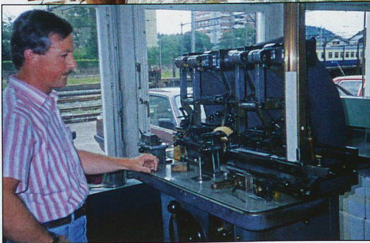
The Edmonson printing machine in Bern SBB.
