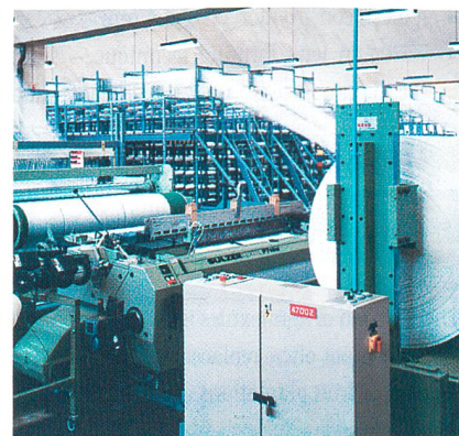
Sulzer Textil Projectile Weaving Machines – weaving tyre cord off a creel behind the machine
