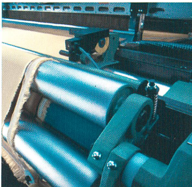
Rapier Weaving Machine – running «Kevlar» at 500 picks / min. at high efficiency
