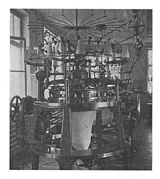
Cotton's knitting machine for knitting stockings, named after the inventor, possesses as many as 32 different appliances called needle-beds. On this machine fashioning is automatic which makes it possible to manufacture fully fashioned stockings.
