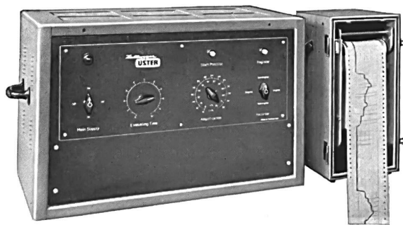
Spectrograph attachment for analysing the yarn readings given by the « Uster » Evenness Tester.
