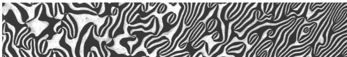
Piezoresponse force microscopy image of the ferroelectric domain structure of multiferroic \text{ErMnO}_3 . The dark and light regions correspond to opposite orientations of the electric dipoles. The vertical dimension is about 20 \mu\text{m} .
