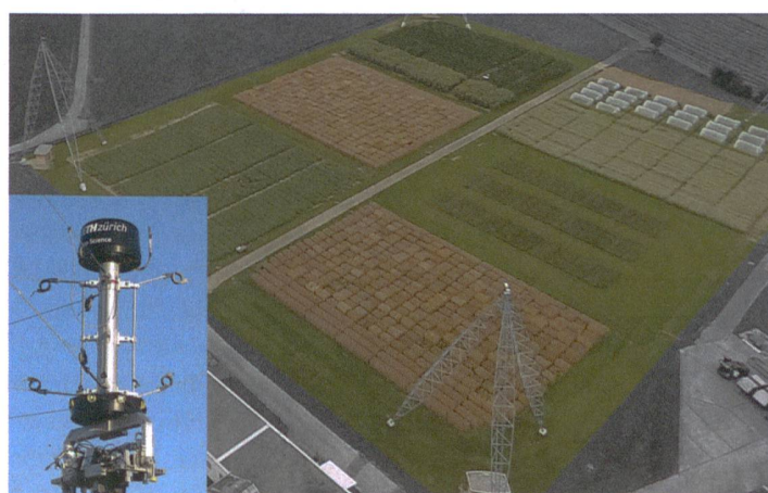
Fig. 3. Field Phenotyping Platform FIP of ETH Zürich. The field site of 1 ha is managed with a crop rotation of forage crops, wheat, soybean, buckwheat and in some years maize, sunflower or oilseed rape. The inset shows the sensor head carrying multiple camera systems. The sensor head is attached to eight ropes guided over the top of the four 24-m-masts in the corners of the field. The length of the ropes is controlled by winches at the bottom of the mast, thereby allowing for precise positioning of the sensor head over the canopy.
