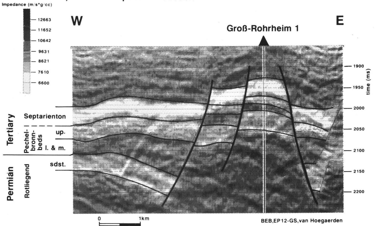
b) schematic geological section
