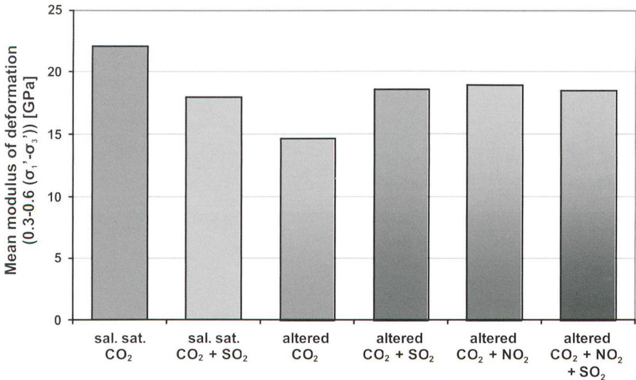
CO<sub>2</sub>-fluid / rock- interaction: Mechanical weakening of the Rotliegend-Sandstone
