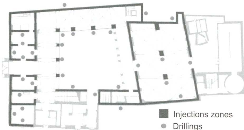
Fig. 2: Above: foundation survey at Palatium Vetus. Below: survey and intervention map.
