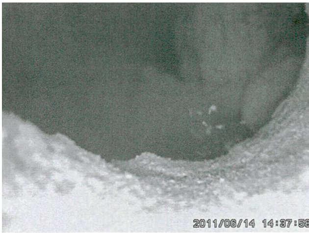
Fig. 13: Cavities in Geneva subsoil.
