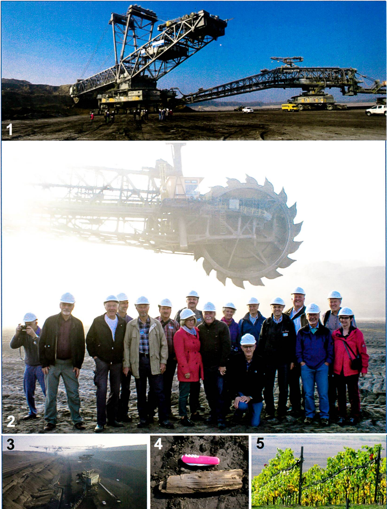
Fig. 3: Welzow-Süd open-cast lignite mine. [1] A bucket-wheel excavator moving on crawlers removes the overburden of the lignite. Cars and participants (with white helmets) for scale (Photo: H. M. Bürgisser); [2] The 17 participants have full confidence in the lignite excavation hardware and technology (Photo: B. Köchel using P. Reichetseder's camera); [3] Current lignite extraction site; bucket-chain excavator in foreground, 500 m long overburden conveyor bridge at the horizon (Photo: U. Seemann); [4] Fossil wood from 2 nd Lusatia Seam (Photo: H. M. Bürgisser); [5] Vineyard at Wolkenberg, on SSW-facing reconstructed slope (Photo: H. M. Bürgisser).
