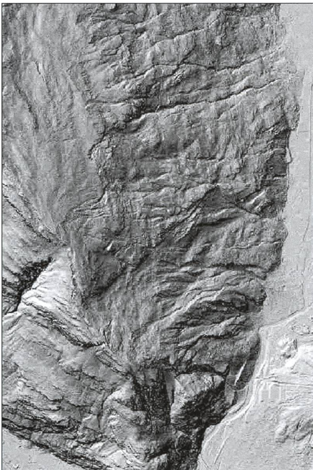
Fig. 2: Shaded relief of a Digital Elevation Model (swissALTI3D copyright 2019 of Swisstopo) and map of the phenomena of the Loderio landslide.
