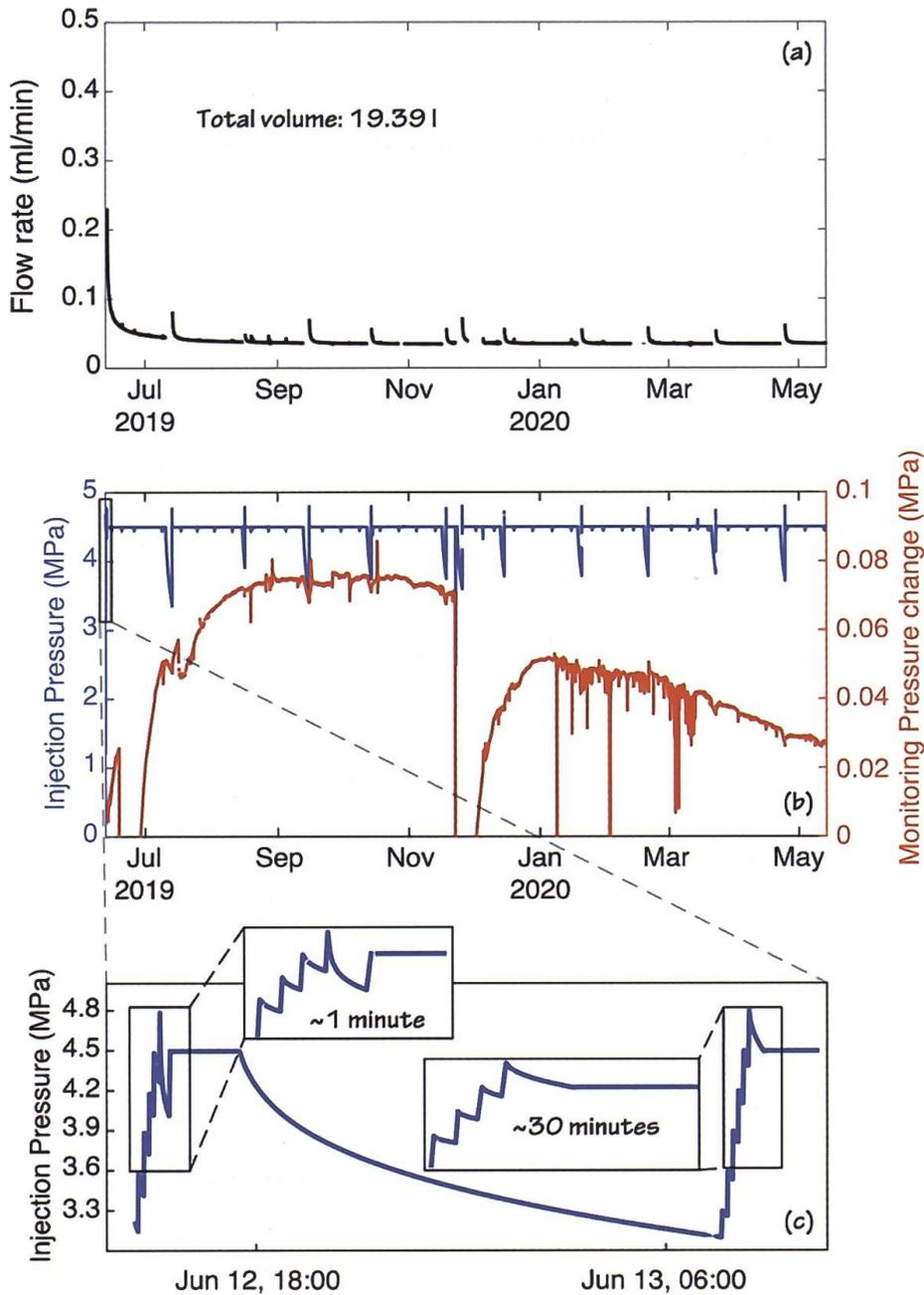
Fig. 13: (a) Flow rate recorded during the one year-long injection of CO<sub>2</sub> saturated fluid. (b) Pressure at injection interval (blue line) and pressure changes recorded at the monitoring interval (red line). See Figure 1b for relative distances. (c) Zoom on injection pressure in the first days of injection.
