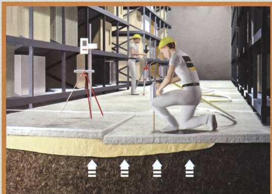
URETEK Floor Lift®
