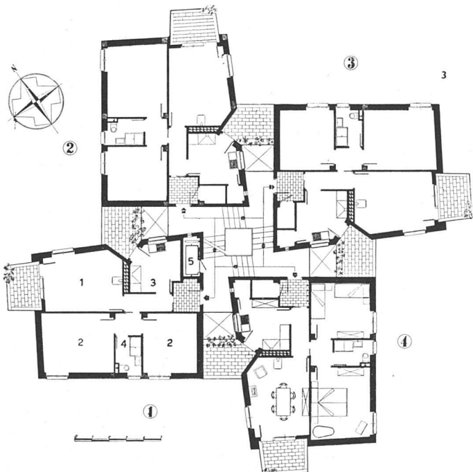
Grundriß eines Turmhauses 1:300 | Plan type d'un immeuble-tour | Typical floor plan of a point house
