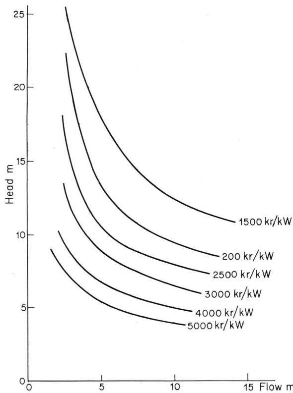
Figure 1. Specific costs of mechanical and electrical equipment for mini power stations. 100 sKr. = 40 sFr. (April 1980).
