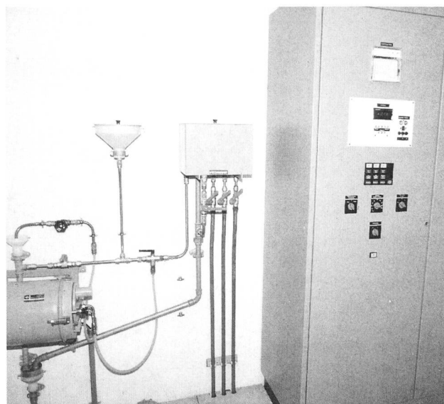
Reference number 3.301. Turbidimeter. Measuring equipment (on the left) for 3 drainage water samples introduced by the 3 supply pipes in the center. The boxes on the right contain the control and monitoring equipment.
