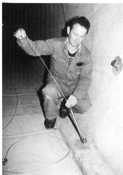
Reference number 1.110-2. Engineer introducing a thermometer in a borehole to measure internal temperature of concrete or roc.
