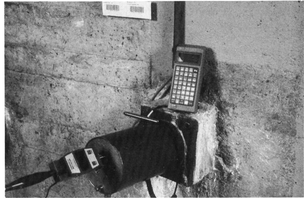
Reference number 2.120-1(2). Rod extensometer for concrete dams. Measuring head for measurements by hand (using a digital dial gauge) and with digital data registration and identification of the measuring points.
