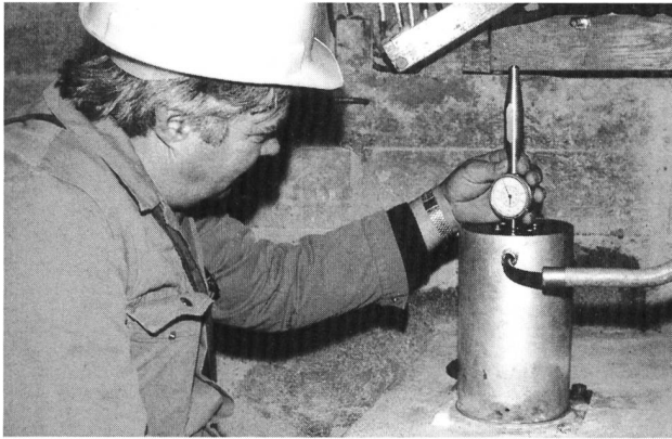
Reference number 2.120-1(1). Rod extensometer for concrete dams. Measuring head with mechanical and electrical reading.
